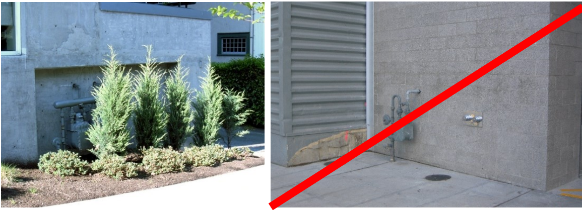
Figure 2.6.A.2 Utility meter location and screening - good and bad examples.
